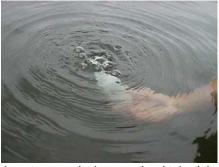
A water sample is properly obtained by lowering the bottle upside down 1-2 feet below the surface, then pointing the bottle up, allowing the bottle to fill (credit: MiCorps staff).
